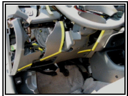
Figure 12. Close-up of damaged knee bolster and instrument panel
