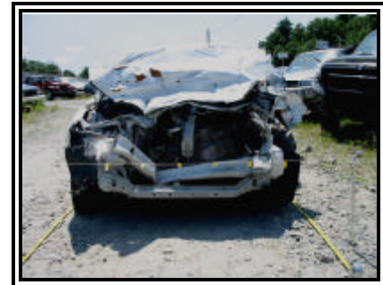
Figure 8. Frontal view of damage to the Honda Civic
