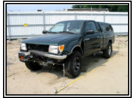
Figure 13. View of frontal damage to the Toyota Tacoma
