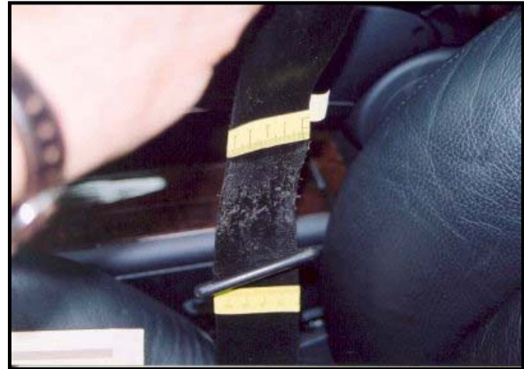
Figure 10: Close-up of the webbing transfer at the latch plate.
