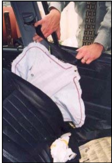
Figure 11: View of the deployed side impact air bag.
