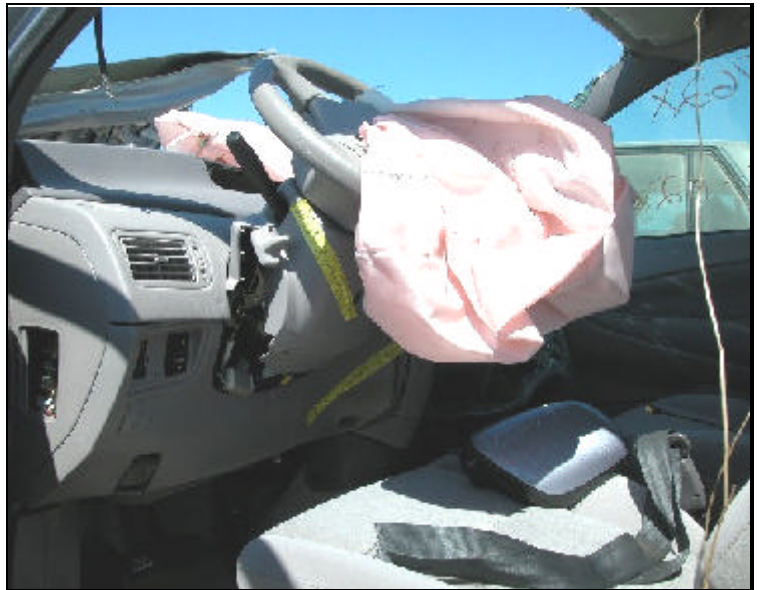
Figure 19. Damage and contact to left side of steering column
