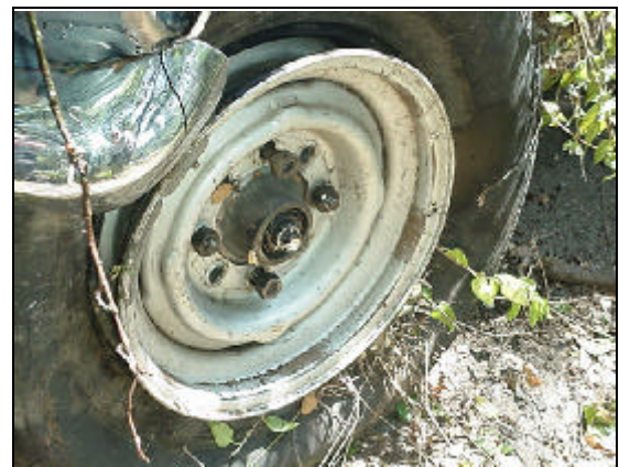
Figure 16. Left front rim (loose and missing lug nuts)
