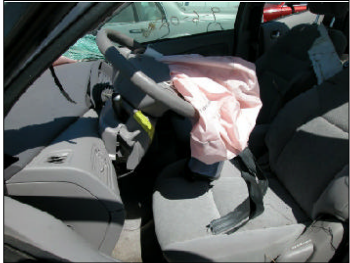
Figure 9. Steering column deformation/air bag
