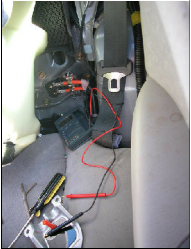
Figure 12. Battery power cable (behind rear seat)
