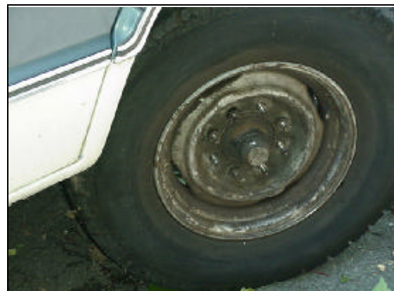
Figure 17. Front right rim (missing and loose lug nuts)
