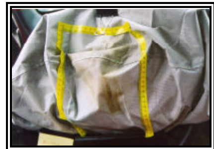
Figure 9. Rear bottom view of the driver's air bag showing the tissue and fabric transfers
