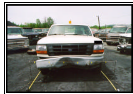
Figure 5. View of frontal damage to the Ford F-150 pickup truck
