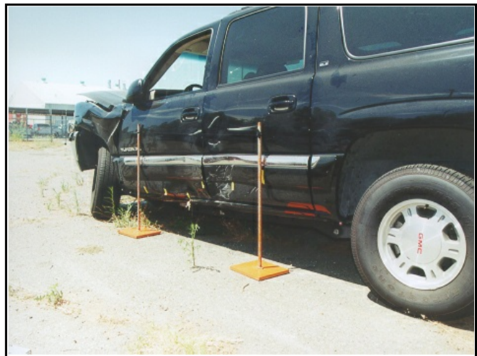
Figure 4. Impact 2, left side damage vs other vehicle.
