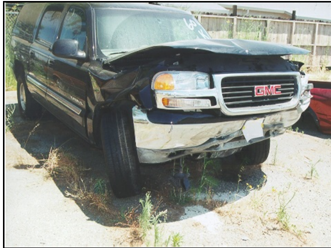
Figure 2. Impact 1, frontal damage vs guardrail.
