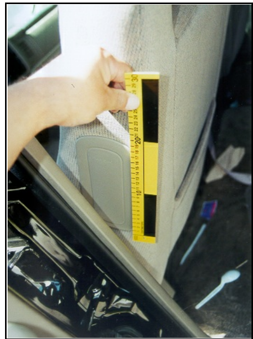
Figure 7. Non-deployed driver's side air bag.
