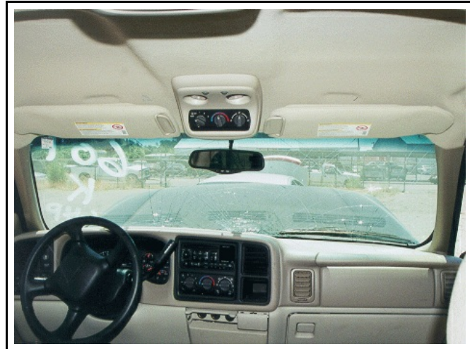
Figure 6. Non-deployed frontal air bags.
