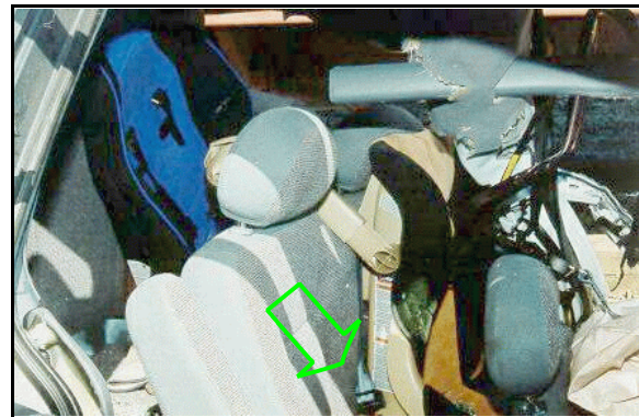
Figure 8: Looking into the case vehicle from the right, second row left CSS and third row left BSS; note, second row left safety belt threaded through CSS frame and buckled (arrow) (case photo #17)
