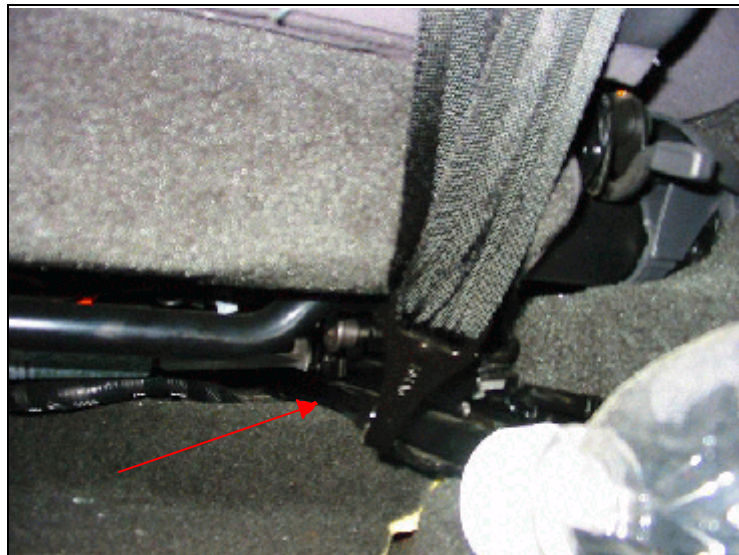
Figure 12. Tether attachment anchorage
