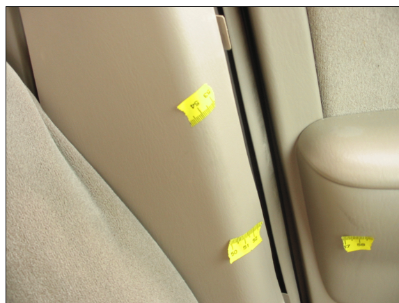
Figure 12: Close-up of occupant contact evidence on interior surface of case vehicle's driver door and left "B"-pillar (case photo #37)
