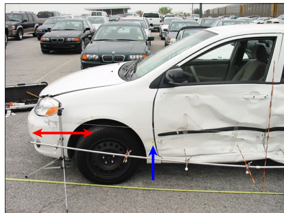
Figure 4: Forward portion of case vehicle's left side impact with contour gauge present; Note: single arrow indicates forward-most location of direct damage and double arrow shows side slap impact to front portion of left fender (case photo #17)
