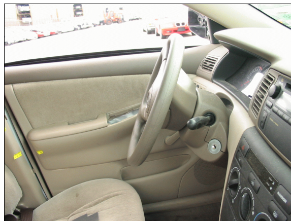
Figure 11: Occupant contact evidence on interior surface of case vehicle's driver door and left "B"-pillar; Note: no movement to steering wheel rim or deployment of driver's air bag (case photo #35)
