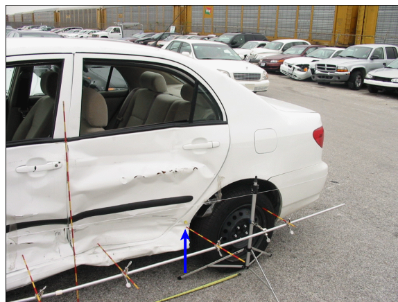
Figure 5: Rearward portion of case vehicle's left side impact with contour gauge present; Note: arrow indicates rear-most portion of direct damage (case photo #18)
