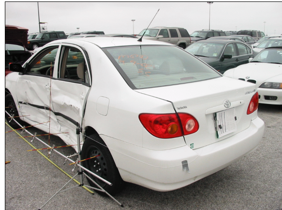
Figure 8: Case vehicle’s left side impact viewed from left of back with contour gauge present (case photo #22a)
