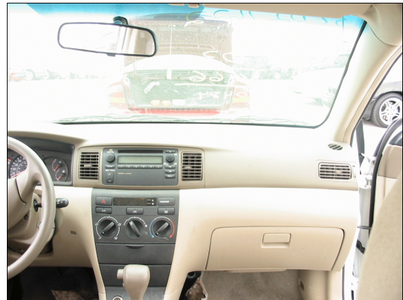
Figure 14: Case vehicle's non-deployed front right passenger air bag and no apparent occupant contact evidence on center and right instrument panel or front right greenhouse areas (case photo #41)
