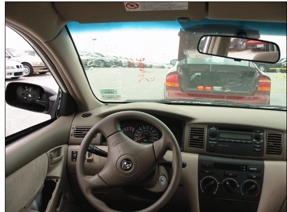
Figure 13: Case vehicle's driver seating area showing non-deployment of driver's air bag and no apparent occupant contact evidence on steering wheel, instrument panel, or greenhouse areas (case photo #39)
