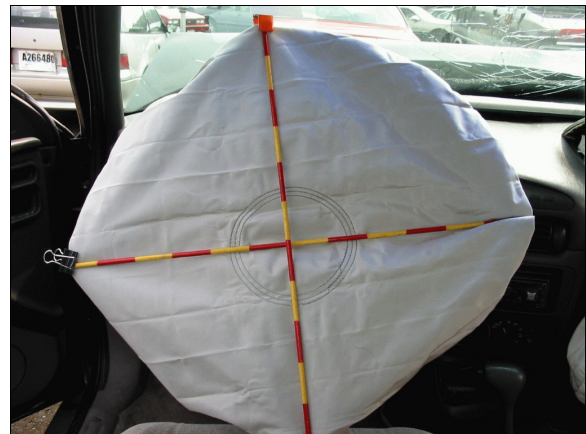
Figure 16: Case vehicle's deployed driver air bag showing no obvious evidence of occupant contact (case photo #47)
