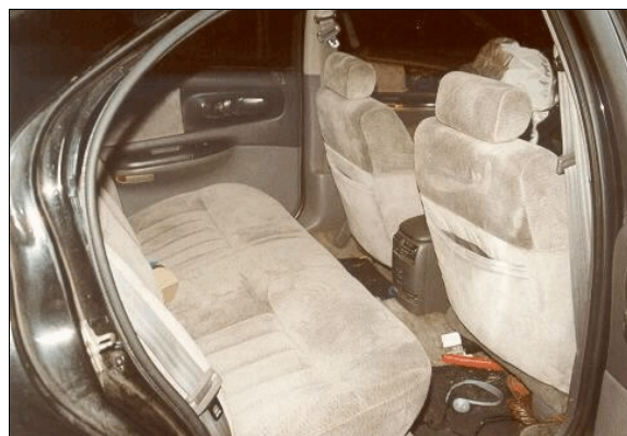
Figure 21: On-scene view of case vehicle's back seating area showing no evidence of occupant contact to back surface of front right passenger's seat back (case photo #78)
