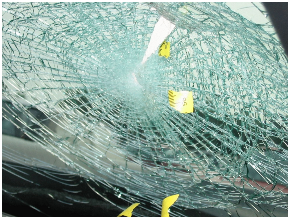
Figure 13: Close-up of contact evidence on case vehicle's right windshield glazing; Note: yellow tape marks strands of hair in glazing (case photo #41)
