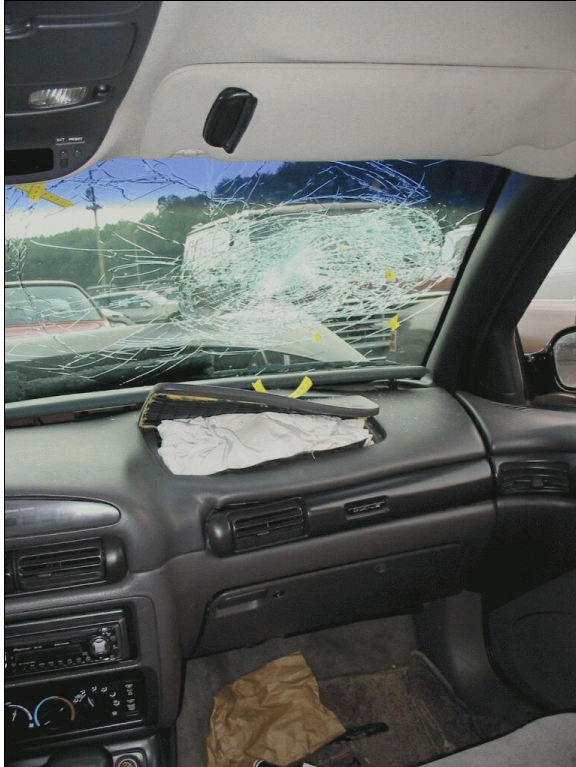
Figure 11: Vertical view of case vehicle's front right seating area showing uneven opening pattern to front right air bag module's cover flap, spider web-type contact to right windshield's glazing, and lack of contact evidence on right sun visor, "A"-pillar, or knee bolster (case photo #38)
