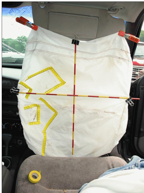
Figure 19: Front surface of case vehicle’s deployed front right passenger air bag showing contact evidence situated along left side of bag’s fabric (case photo #52)
