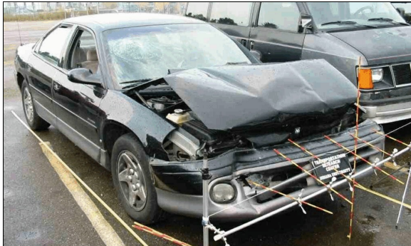
Figure 4: Case vehicle's bumper and above bumper frontal damaged viewed from right of front with contour gauge positioned along top of bumper (case photo #28)
