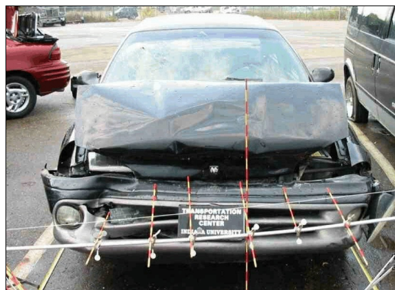
Figure 8: Case vehicle's front bumper and above bumper damage with contour gauge positioned at top of bumper's fascia (case photo #07)
