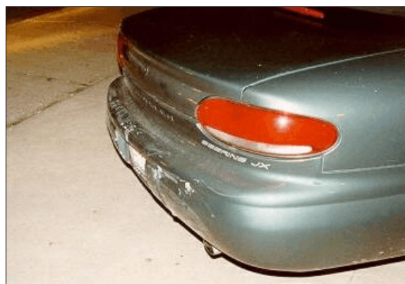
Figure 23: On-scene view of Chrysler's rear bumper viewed from right back showing contact evidence across bumper's fascia from impact with case vehicle (case photo #80)
