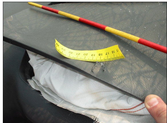
Figure 18: Close-up of case vehicle front right passenger air bag module's cover flap showing cut near front edge of flap (case photo #67)
