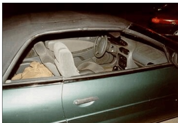
Figure 22: On-scene view of Chrysler's interior showing non-deployed driver and front right air bags (case photo #81)
