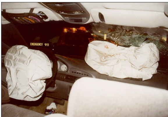
Figure 6: On-scene view of case vehicle's deployed driver and front right passenger air bags; Note: cracked right windshield glazing above front right air bag's fabric (case photo #76)
