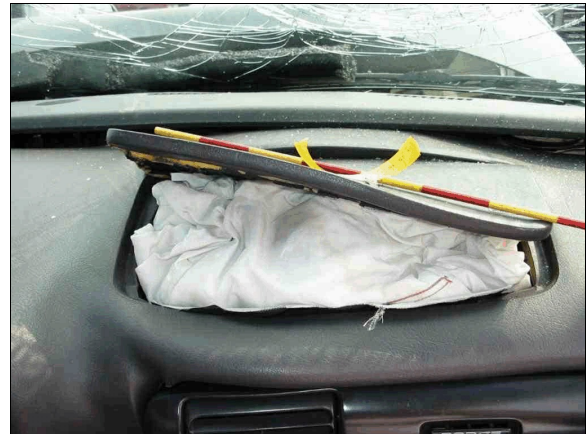
Figure 17: Close-up of case vehicle's front right passenger air bag module showing distortion to module's cover flap caused by uneven opening (case photo #68)
