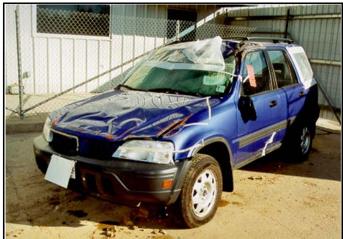
Figure 9. Exterior damage to case vehicle-left side.
