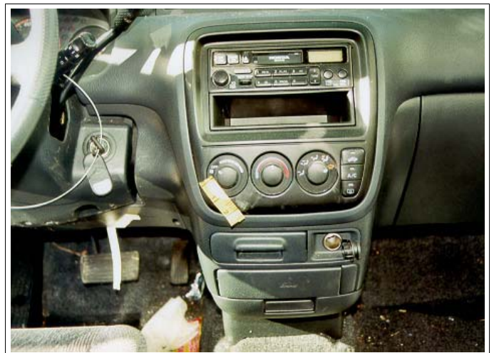
Figure 12. Damaged left and center instrument panel.
