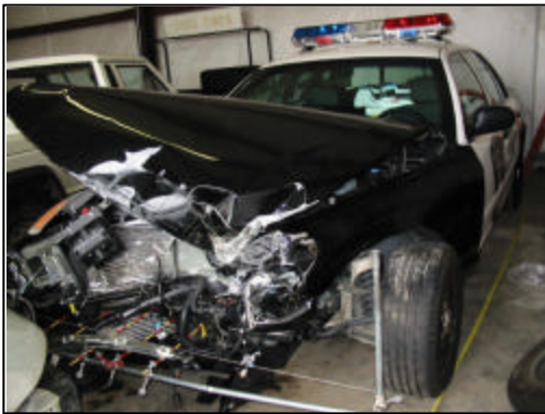
Figure 4. Front left view of damaged Crown Victoria
