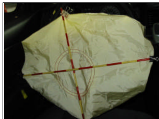
Figure 10. View of the deployed driver's air bag
