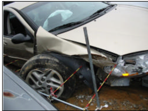
Figure 8. Close-up of right front damage
