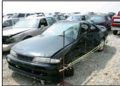
Figure 8. Left side damage of Nissan.
