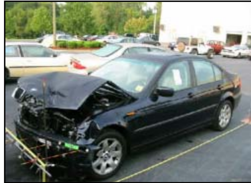
Figure 5. Front damage, BMW.
