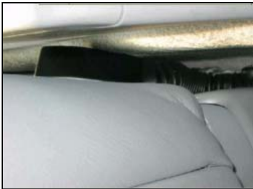
Figure 9. Actuated front left safety belt pretensioner.
