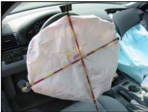
Figure 6. Driver's facial contact to air bag.
