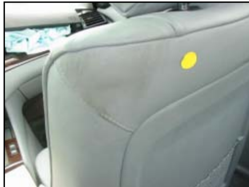
Figure 14. Rear right occupant contact to rear of front right seat back.
