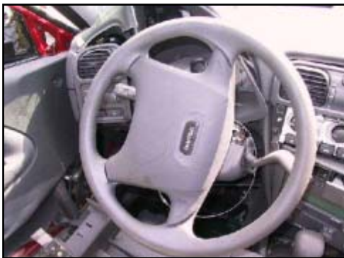
Figure 11. Non-deployed driver's frontal air bag.
