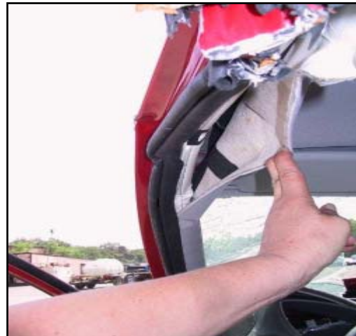
Figure 10. Non-deployed curtain in left roof side rail.
