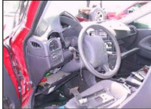
Figure 7. Interior damage from intrusion.
