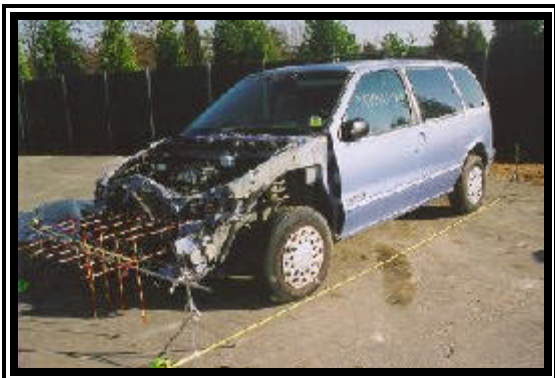
Figure 2. Front left damage to the 1997 Nissan Quest XE.
