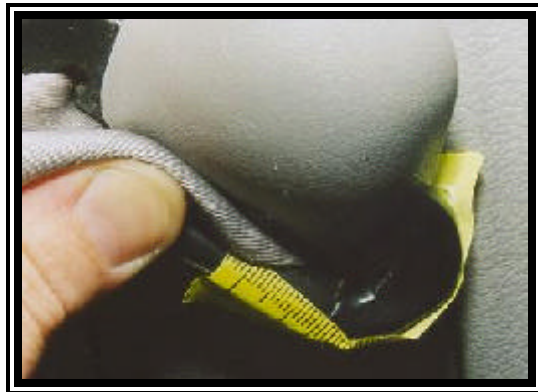
Figure 6. Loading marks to the D-ring of the driver restraint.
