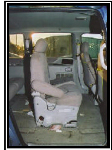
Figure 11. Deformation to the second row seat back.
