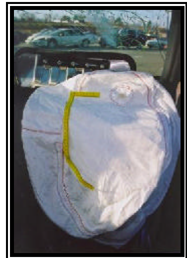
Figure 10. Contact evidence to the left side aspect of the passenger air bag.
