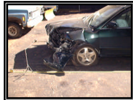
Figure 7. Left side view showing maximum crush and displaced left front wheel
