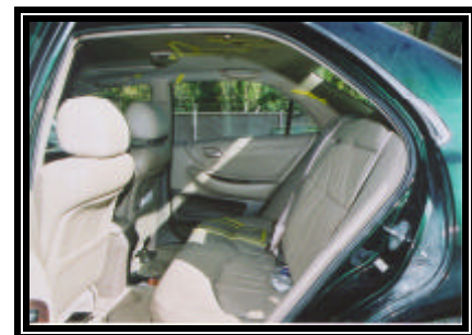
Figure 10. View of rear seat showing intruded seat back
