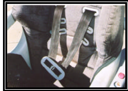
Figure 16. View of the harness straps and retainer clip
