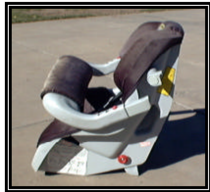
Figure 17. View of the fractured left arm of the child safety seat
