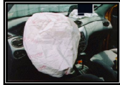
Figure 14. Driver's redesigned air bag
