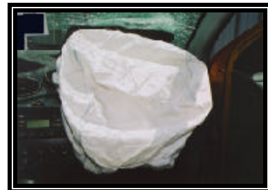
Figure 15. Redesigned front right passenger's air bag
