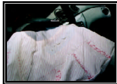
Figure 13. Driver's redesigned air bag showing vent ports and stitching
