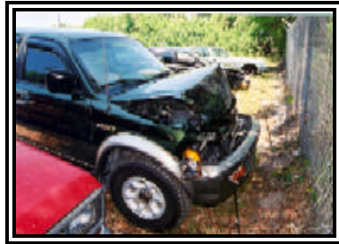
Figure 4. Full frontal damage to the Mitsubishi.
