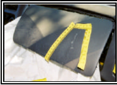
Figure 11. Scuff with tissue transfer to the module cover flap.
