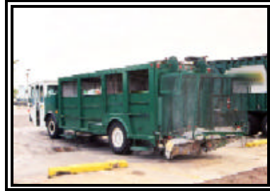
Figure 5. Damage to the rear basket of the recycler truck.
