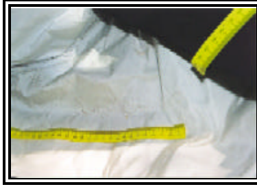
Figure 12. Tissue transfers on the top panel of the front right air bag.
