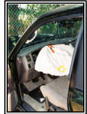
Figure 15. Trajectory of the driver into the deploying air bag and steering assembly.
