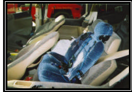
Figure 5. Front seat back deflection
