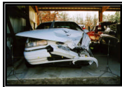
Figure 10. Frontal damage to 1993 Ford Taurus
