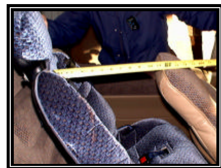
Figure 12. View showing distance between the booster seat and the damaged driver's seat back
