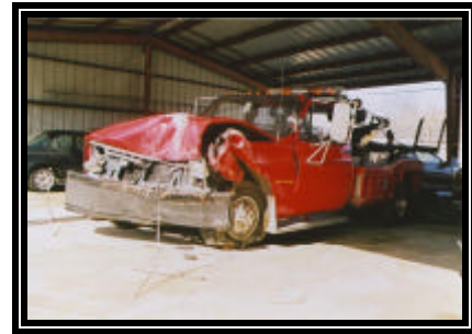
Figure 9. Frontal damage to 1985 Chevrolet tow truck
