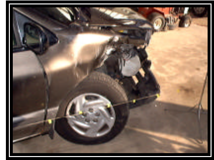
Figure 4. View of right front side damage to the Caravan
