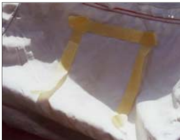
Figure 14: Close-up of skin transfer area on front portion of top surface of case vehicle's front right passenger air bag (case photo #30)
