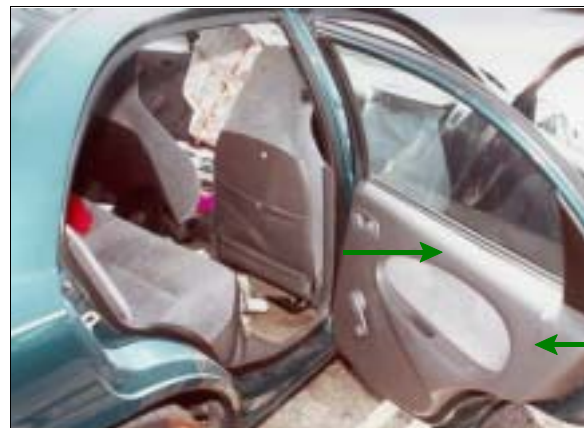
Figure 10: Case vehicle's deformed front right seat back from contact by back right passenger; Note: blood (arrows) on window sill and door panel (case photo #35)
