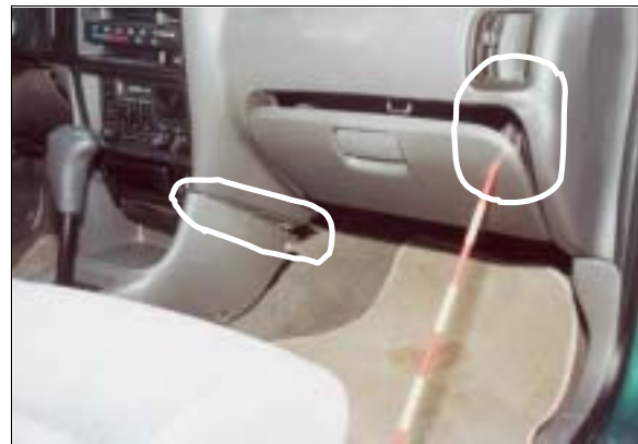
Figure 9: Case vehicle's front right passenger seating area showing right knee contact to glove box and right instrument panel; Note: center floor mounted console also ajar (case photo #32)
