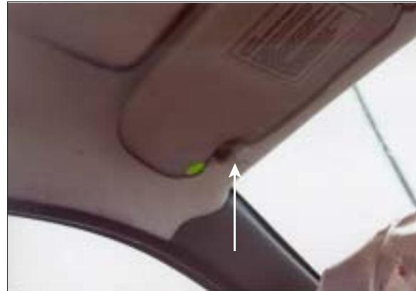
Figure 8: Case vehicle's driver sun visor showing hair clump on sun visor's stem from contact with driver's scalp (case photo #23)
