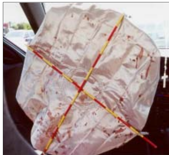
Figure 12: Case vehicle's driver air bag showing copious blood smears from driver's scalp injuries (case photo #24)
