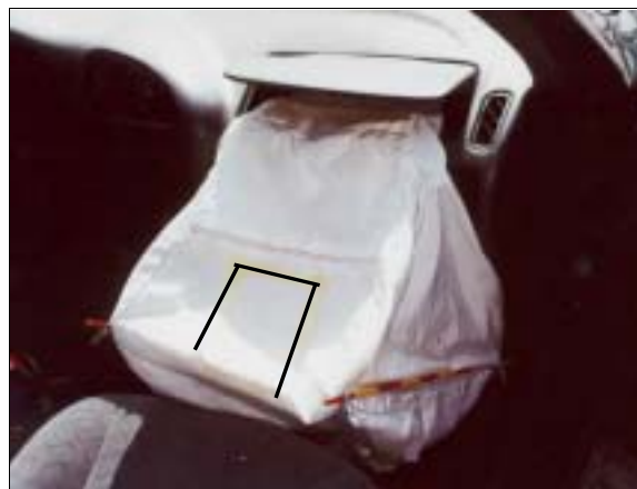
Figure 13: Skin transfer area on front portion of top surface of case vehicle's deployed front right passenger air bag (case photo #29)
