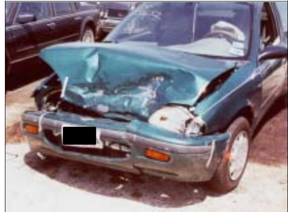
Figure 2: Case vehicle's damaged front viewed from left of front with bumper fascia placed on bumper; Note: tape indicates width of direct damage (case photo #11)
