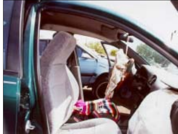
Figure 11 Case vehicle's front seating area showing deformation to front right seat back from contact by back right passenger and deployed frontal air bags (case photo #26)
