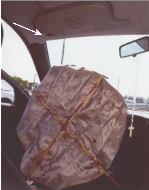
Figure 7: Vertical view of case vehicle's driver air bag and header area showing contact (arrow) to sun visor post (case photo #25)
