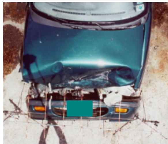
Figure 6: Overhead view of case vehicle’s frontal damage with contour gauge present; Note: bumper fascia lying on ground (case photo #12)
