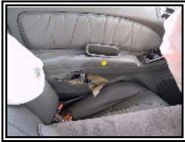
Figure 3. Driver's left hip loading to the left door armrest.
