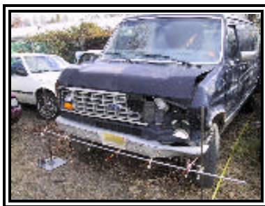
Figure 5. Frontal damage to the Ford Econoline.
