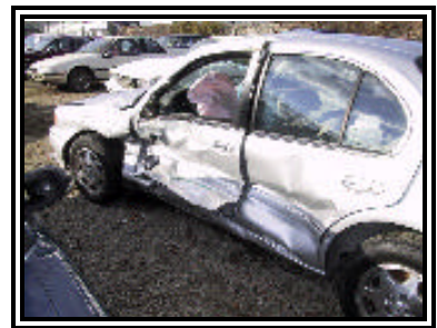
Figure 2. Exterior damage to the Infinity I30.
