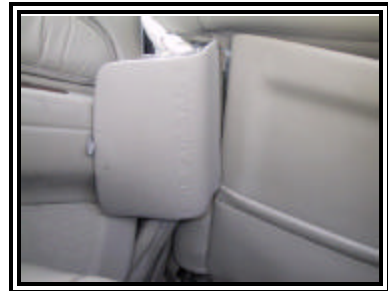
Figure 8. Side air bag cover flap opening to rear of vehicle
