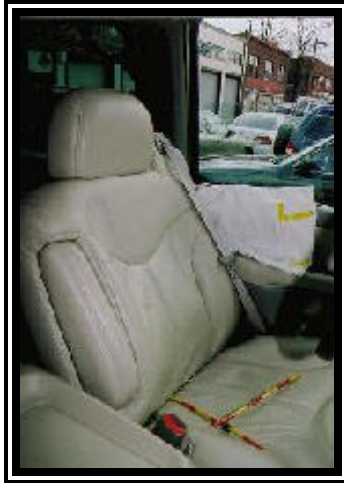
Figure 11. 2001 GMC Yukon XL deployed side impact air bag.
