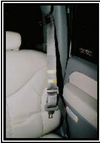
Figure 7. Loading marks to the second row left shoulder belt webbing.
