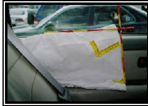
Figure 12. Close-up view of the deployed side impact air bag.
