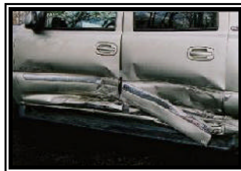
Figure 4. Close up view of the direct contact damage.
