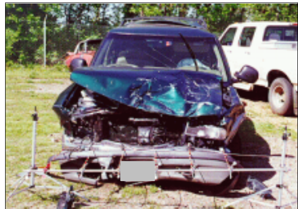
Figure 3: Case vehicle's frontal damaged from impact with Mazda's right side with contour gauge present (case photo #12)
