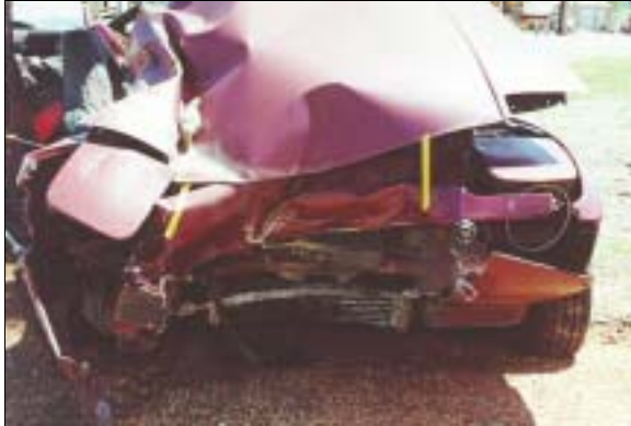
Figure 8: Mazda's frontal deformation from pole impact; Note: tape indicates width of direct damage (case photo #37)
