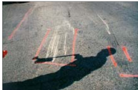
Figure 6: Close-up on-scene view looking north at Mazda's left front tire (right) and undercarriage scraping (center) on asphalt surface at maximum engagement (case photo #50b)
