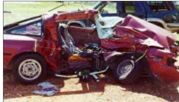
Figure 4: Mazda's struck right side; Note: tape indicates width of direct damage (case photo #44)
