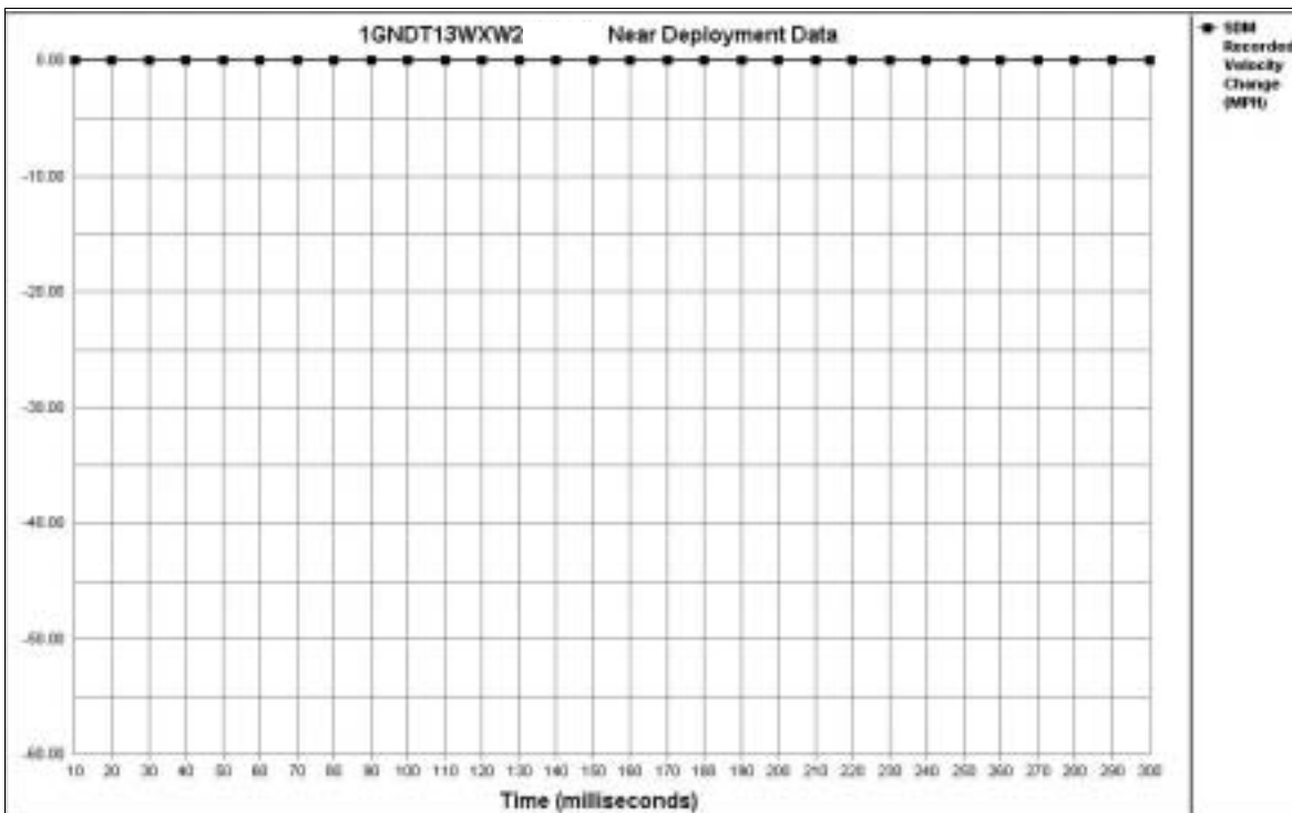
Figure 23: The case vehicle sustained a velocity change of approximately 0 km.p.h. (0 m.p.h.) during the entire 300 milliseconds recorded after the near deployment was detected
