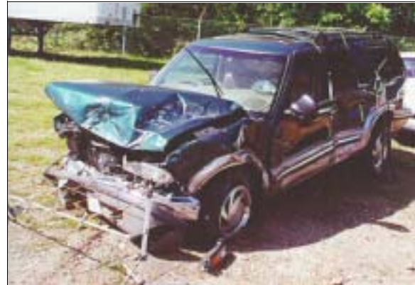
Figure 13: Case vehicle’s front and left side damage viewed from left of front; Note: pole impact to left rear door and side slap impact to left back (case photo #17a)
