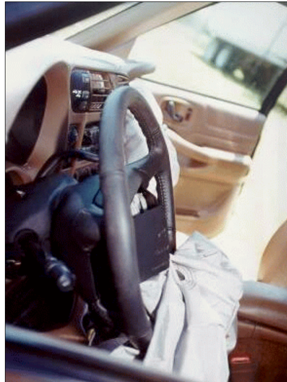
Figure 15: Case vehicle's steering wheel showing bending to the top portion from occupant loading (case photo #31)
