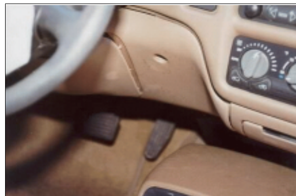
Figure 16: Case vehicle's driver knee bolster on right side of steering column showing scuff and deformation from driver's knee (case photo #33)
