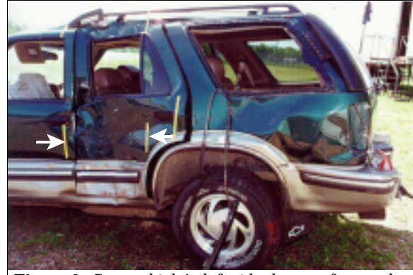
Figure 9 Case vehicle's left side damage from pole (vertical tape and arrows) and side slap impact to left back from Mazda (case photo #20)
