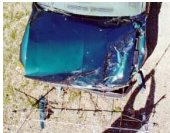
Figure 7: Overhead view of case vehicle's frontal deformation from impact with Mazda's right side; Note: damage atop hood from Mazda's right front door and quarter panel (case photo #13)
