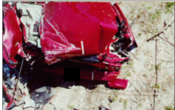
Figure 8: Overhead view of case vehicle's severe frontal damage with contour gauge present; Note: front has narrow field "L" that faces primarily downward (case photo #09)
