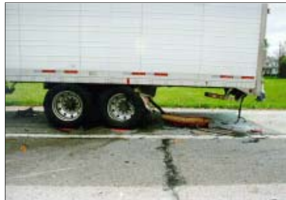
Figure 20: On-scene view looking southward at struck trailer showing trailer's underride damage and case vehicle's forward penetration to left rear tandem wheels; Note: rim damage to trailer's left back outside wheel (case photo #48)
