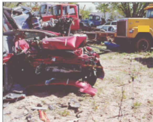
Figure 3: Reference line view from right showing case vehicle's severe frontal deformation and rightward end displacement (case photo #11)
