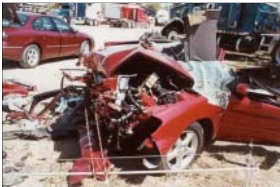
Figure 9: Frontal view of damage to case vehicle's front with contour gauge present; Note: narrow field "L" because front end was displaced almost 90 degrees to the right (case photo #08)
