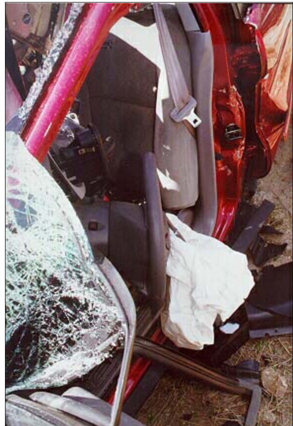
Figure 19: Case vehicle's steering wheel and driver air bag viewed while looking rearward down left side of vehicle (case photo #27)
