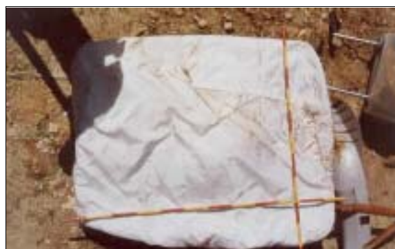
Figure 17: Front surface of case vehicle's front right passenger air bag showing discoloration to air bag's fabric as a result of crash (case photo #36)
