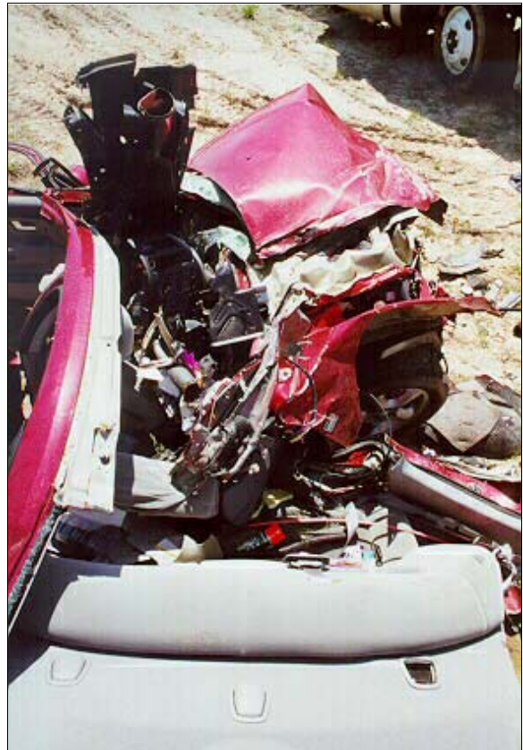
Figure 10: Overhead view of case vehicle's severe frontal deformation and intrusion; Note: photo taken while standing on trunk (case photo #40)
