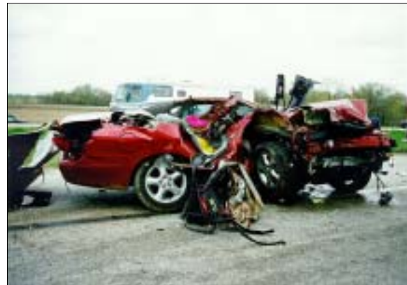
Figure 6: On-scene view of case vehicle at final rest, straddling the inside eastbound lane heading southeastward; Note: roof peeled back from severe underride damage (case photo #49)
