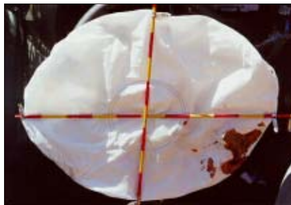
Figure 15: Case vehicle's driver air bag showing only a blood transfer on air bag (case photo #32)
