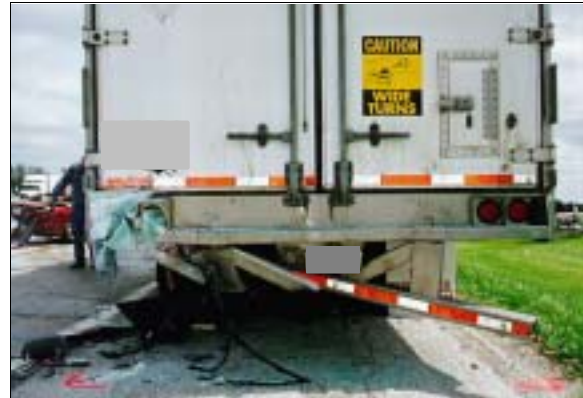
Figure 4: On-scene view looking east at damage to stopped trailer's back surface and underride guard (case photo #43)
