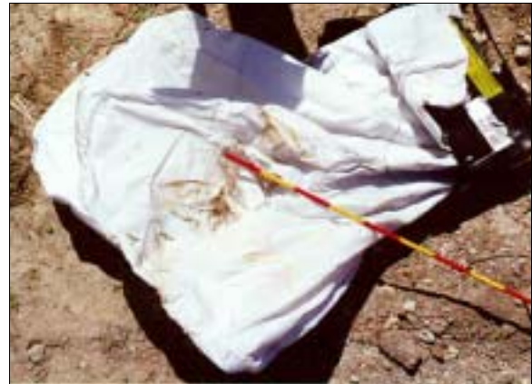
Figure 18: Case vehicle's deployed front right passenger air bag and removed air bag module showing tear to vent port (case photo #35)
