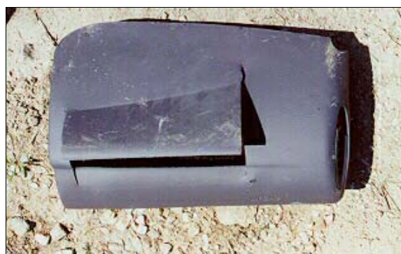
Figure 16: Close-up of case vehicle's right instrument panel which was torn off during underide of trailer; Note: front right air bag module's cover flap (case photo #38)
