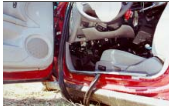
Figure 11: Intrusion and deformation to case vehicle's lower instrument panel and knee bolster for driver's seating area (case photo #25)
