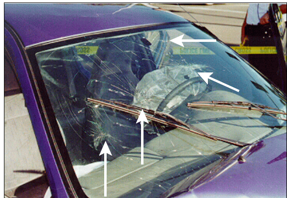
Figure 4: On-scene view of cracks in case vehicle's windshield glazing (case photo #16)
