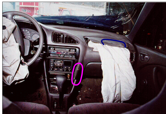
Figure 6: Case vehicle's instrument panel, deployed air bags and center console; Note: scuffs on front right air bag module's cover flap and scuffed and cracked center console (case photo #19)
