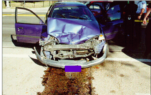
Figure 3: On-scene view of case vehicle's front damage at final rest; Note: front bumper fascia on ground and radiator fluid spill (case photo #07)
