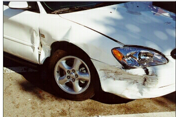
Figure 7: On-scene front of left view of damage to Ford's right front from impact with case vehicle; Note: direct damage begins near right front corner (case photo #31)
