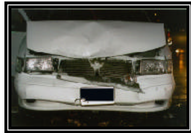
Figure 6. Frontal damage showing damage from the Pathfinder's spare tire
