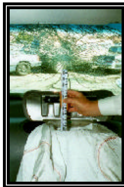
Figure 8. Interior view showing windshield strike
