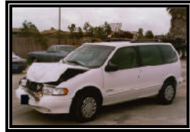
Figure 5. Damage to the Nissan Quest
