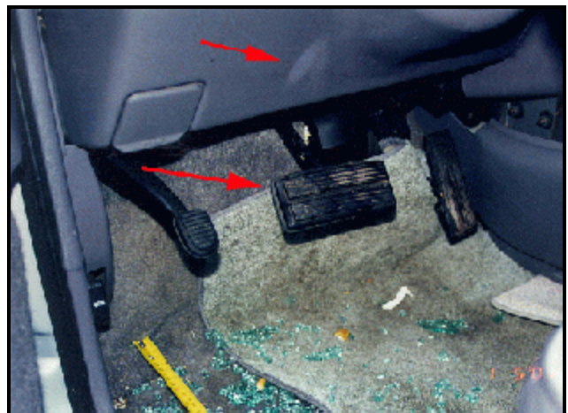
Figure 16. Left knee contact/deformed brake pedal 11
