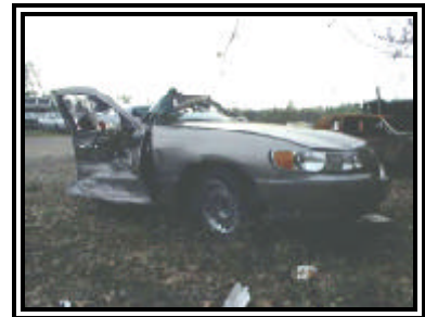
Figure 5. Right front damage to the Town Car
