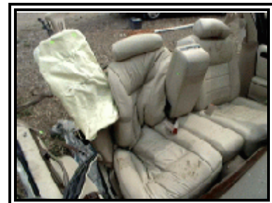
Figure 8. Displaced front seating positions in the 2000 Lincoln Town Car
