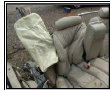
Figure 11. Deployed right front passenger's side air bag
