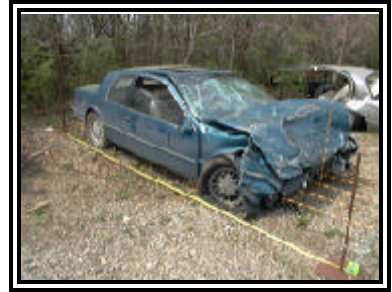
Figure 9. Frontal damage to the 1993 Mercury Cougar
