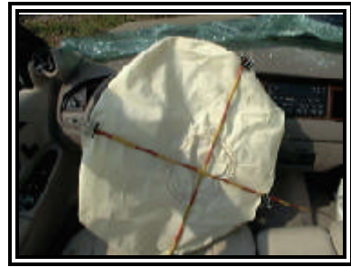
Figure 10. Deployed redesigned driver's air bag
