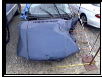
Figure 8. Damage from utility pole impact
