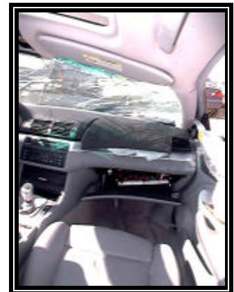
Figure 10. Multiple passenger compartment intrusions
