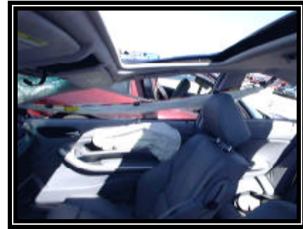
Figure 15. Deployed right front side air bag and right HPS
