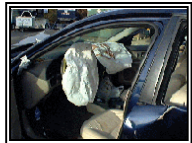
Figure 10. Overall view of the deployed frontal air bags in the Ford Taurus.
