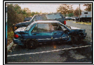
Figure 9. Front and rear impact damage to the right side of the Tracer.
