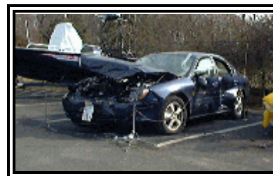
Figure 1. Front and side damage to the 2000 Ford Taurus.
