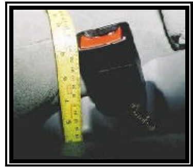
Figure 8. Pretensioner deployment in the front right restraint buckle.
