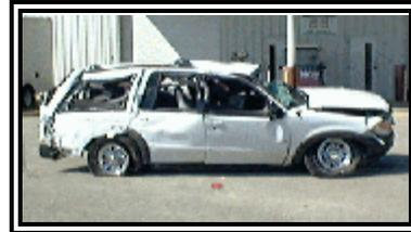
**Figure 10. Right side rollover damage.**
