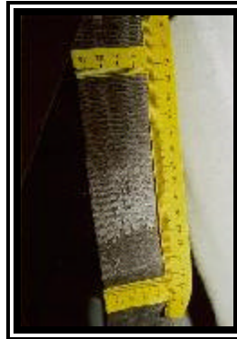
Figure 8. Loading marks to the front left shoulder belt webbing.
