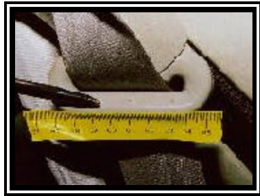
Figure 7. Abrasions to the front left restraint D-ring.
