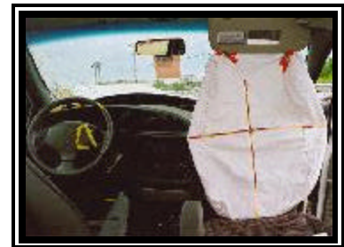
Figure 9. 1996 Dodge Caravan SE non-deployed driver air bag and deployed passenger air bag.
