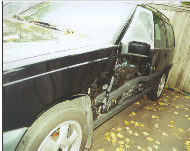
Figure 2. Left side damage to case vehicle.
