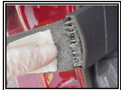
Figure 5. Partial separation of the right front lap belt energy management loop.
