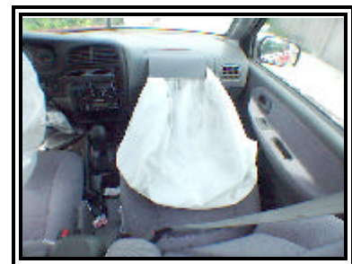
Figure 7. Deployed mid mount front right passenger air bag.
