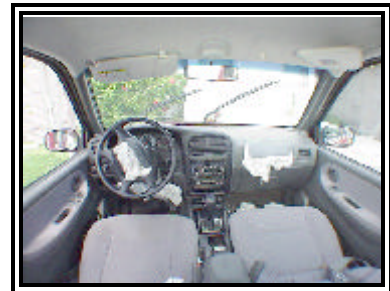
Figure 4. Overall view of the frontal air bag system and the Kia's interior.
