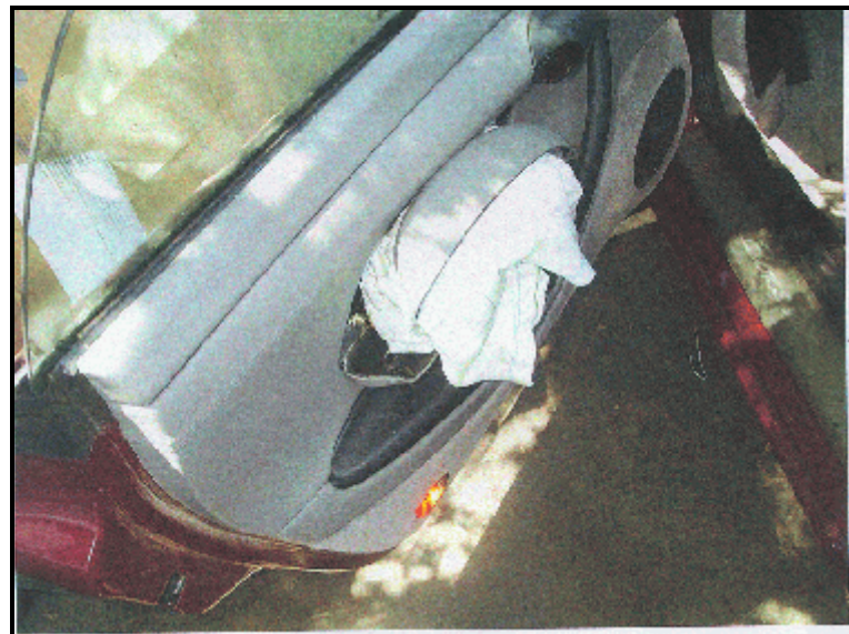
Figure 5. Driver's door mounted side air bag
