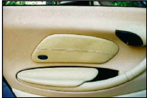
Figure 3. Exemplar view of driver's door mounted side air bag
