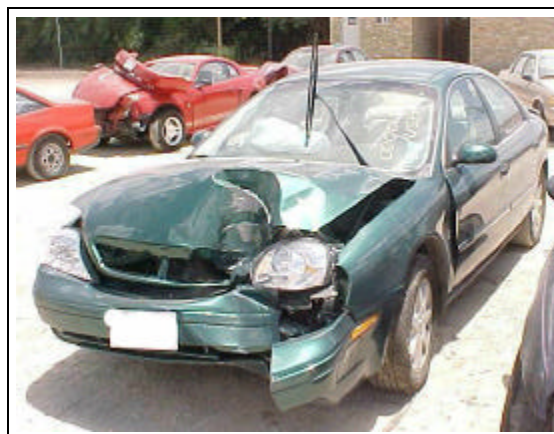
Figure 4. Exterior front damage to case vehicle
