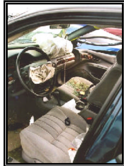
Figure 5: Interior view depicting the forward track position of the right seat.
