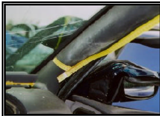
Figure 8: Discharge spray on the right A-pillar.
