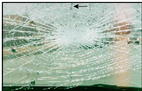
Figure 7: Case vehicle's windshield struck by the front right passenger; Note: arrow points to hair transfer (case photo #20)
