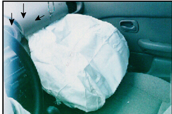
Figure 6: Case vehicle's front right passenger air bag; Note: arrows point to possible occupant contact areas (case photo #21)
