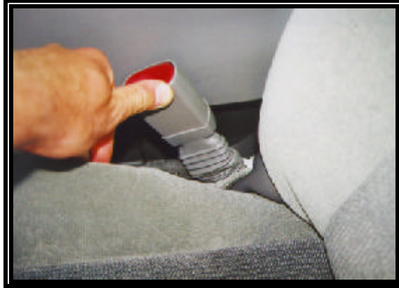
Figure 7: View of the left inboard buckle anchor.
