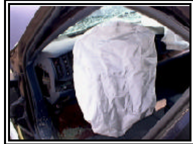
Figure 7. Redesigned driver's air bag
