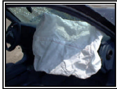
Figure 8. Redesigned front right passenger's air bag
