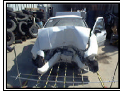
Figure 6. Frontal damage to Ford Tempo
