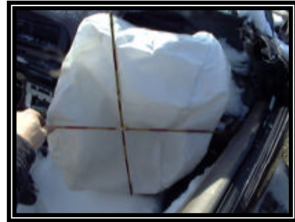
Figure 10. Redesigned front right passenger's air bag
