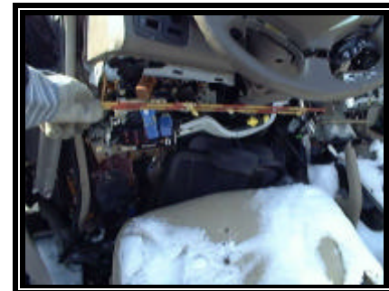
Figure 7. Intruded left toe pan and left instrument panel
