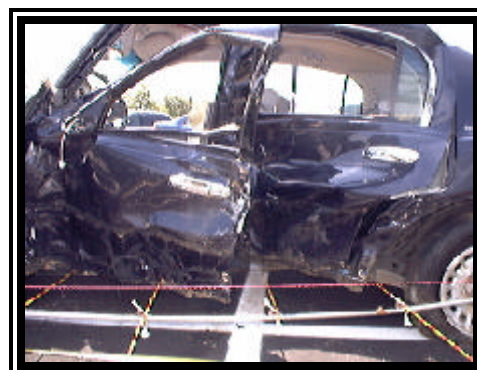
Figure 5. Overlapping damage to the left side surface.
