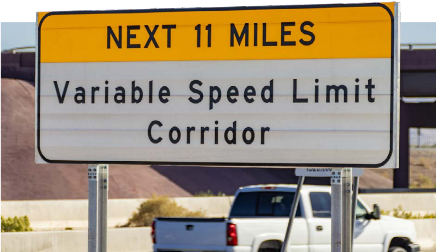
A roadside sign alerts motorists to the variable speed limit corridor that is part of the dust detection system on I-10 between Phoenix and Tucson.
