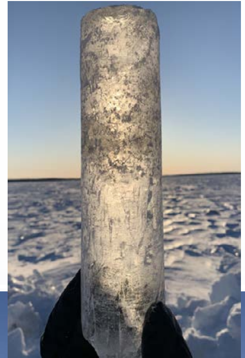
Taking a core sample of ice, like this one from the Tanana Ice Bridge, provides information about the quality and type of ice in addition to measuring the thickness.
