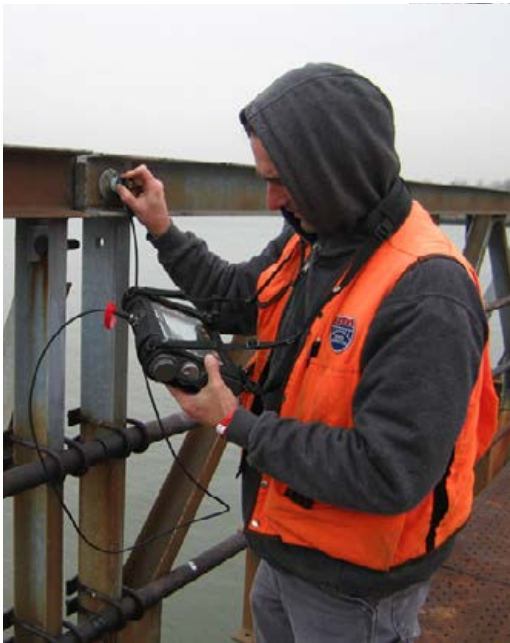
Inspectors perform ultrasonic testing, a nondestructive evaluation technique, on two bridges.
