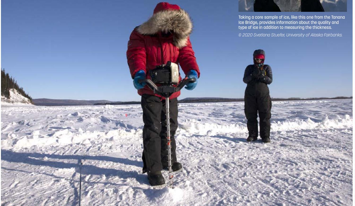
The thickness of the ice can be measured using an auger, as shown here, but this method enables monitoring only at individual locations.
