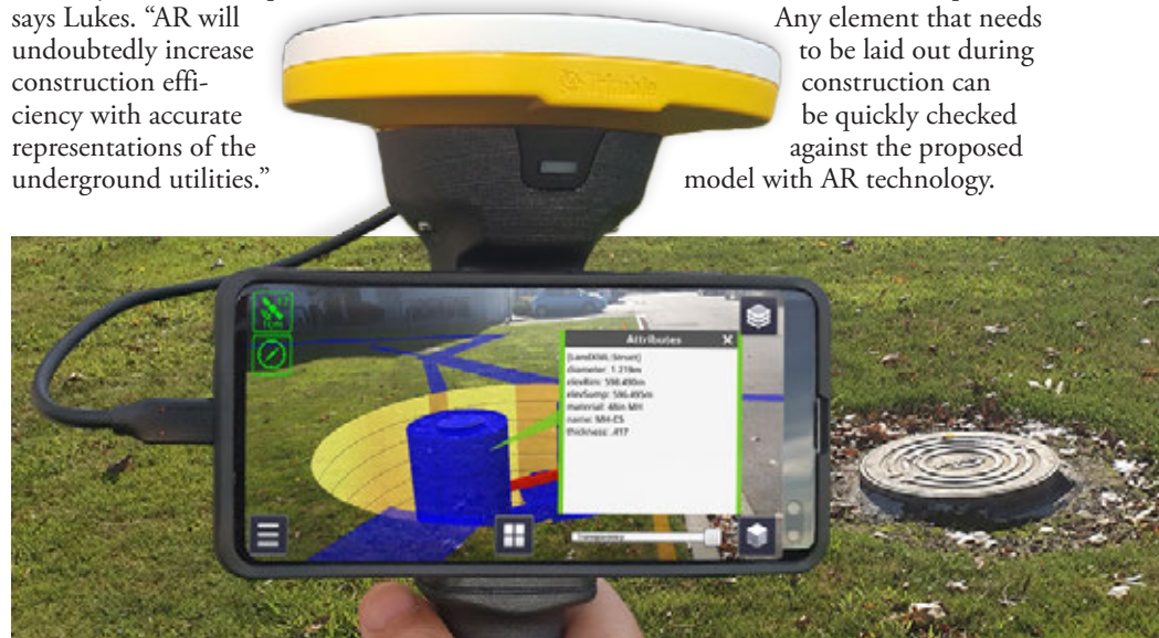
AR devices can provide a 3D virtual view of underground utilities, such as this manhole access point and the surrounding piping, as well as text with associated data.
