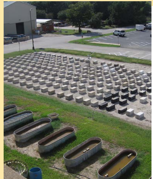
Outdoor exposure sites for durability testing at the University of Texas at Austin. © Racheal Lute.
