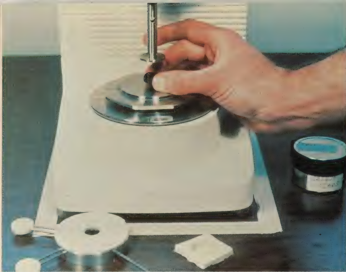
The SHRP dynamic shear rheometer measures the stiffness of an asphalt binder.
