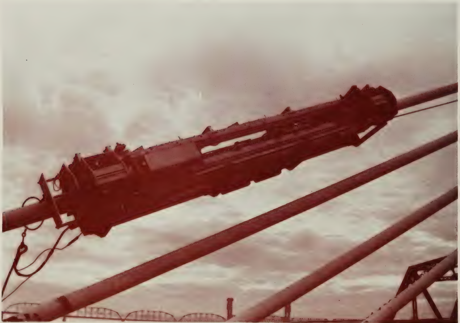
Figure 2.—Prototype MPC on stay-cable Pasco-Kennewick Intercity Bridge over the Columbia River, Washington.
