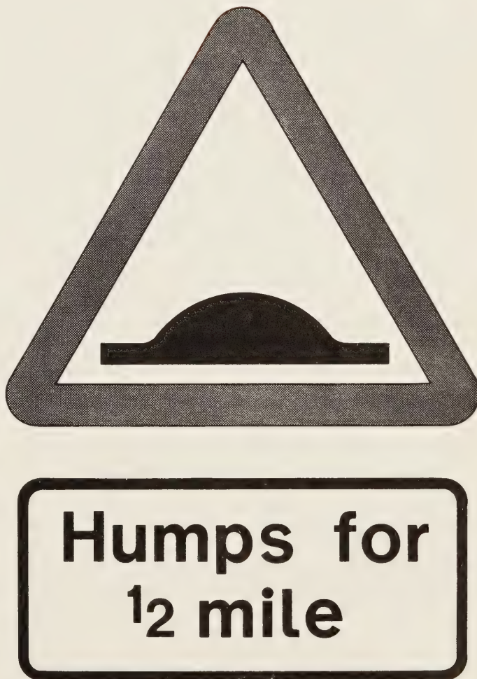
Figure 6.— Symbolic sign and supplementary plate in conjunction with road humps in the United Kingdom. (10)
