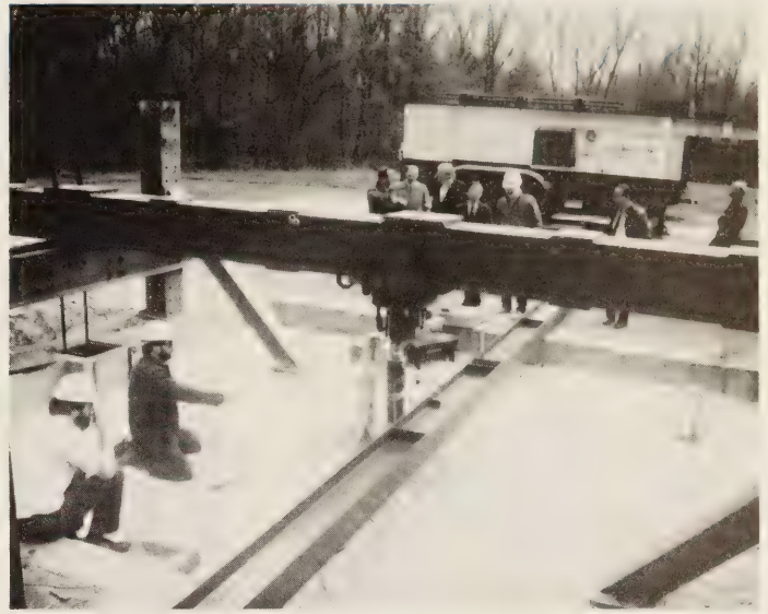
Load test on a one-quarter scale fully instrumented model timber pile in an outdoor sand test pit.
